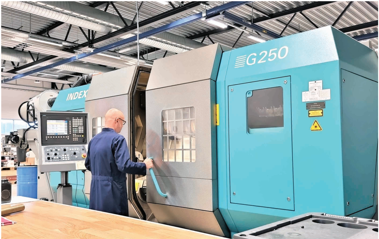
Multi spindle lathe with 5 axes milling capabilities
