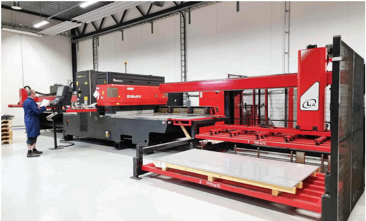
Laser cutting of stainless steel parts
