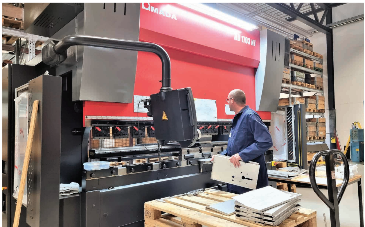
8 axes 170t automatic press brake for processing sheet metal parts
